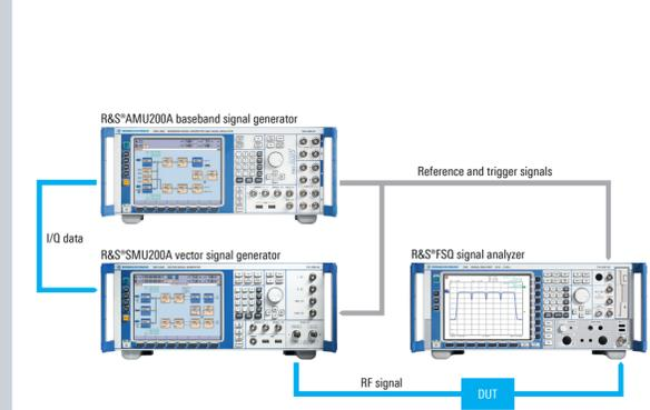
For example, up to four component carriers with 20 MHz bandwidth each are conveniently aggregated to a bandwidth of 80 MHz by means of the R&S SMU200A and R&S AMU200A signal generators which feature a two-path concept.
