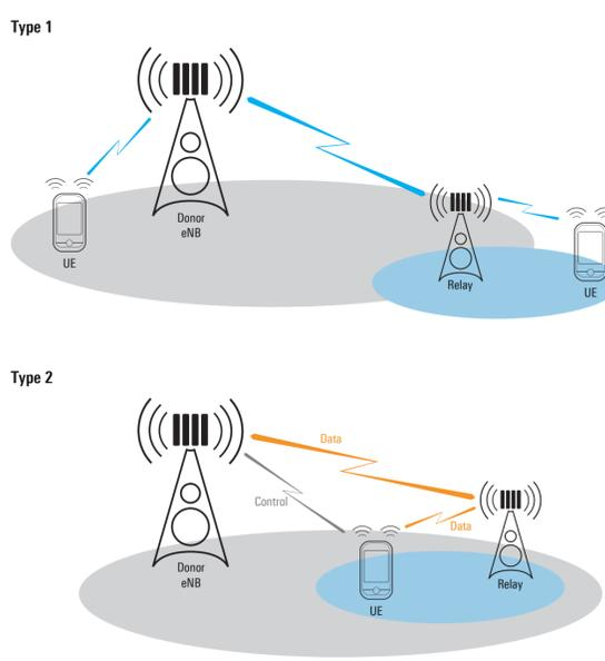
Relaying enhances coverage and capacity. The UEs communicate with the relay node, which in turn communicates with a donor eNB.
