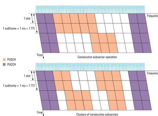
Single carrier frequency division multiple access (SC-FDMA) is maintained as the basic LTE-Advanced uplink transmission scheme.
