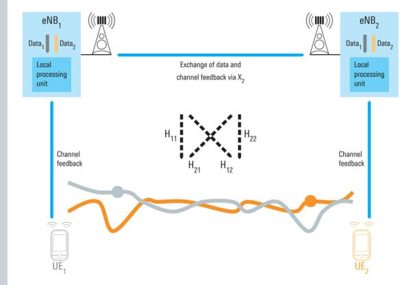
CoMP aims to turn the inter-cell interference into a useful signal specifically at the cell border.
